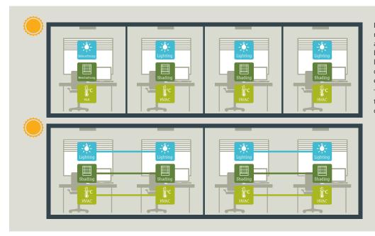
Desigo Room Automation offers maximum flexibility. With its advanced segment concept, the building floor plan and the room layout can be adjusted easily and quickly – without modifying electrical or HVAC installations.
