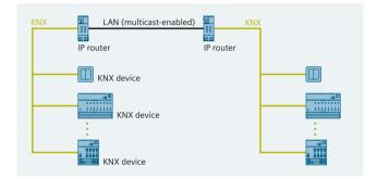
The new KNXnet/IP standard enables KNX telegrams to be transmitted via Ethernet (LAN), which leads to new applications and solutions.
