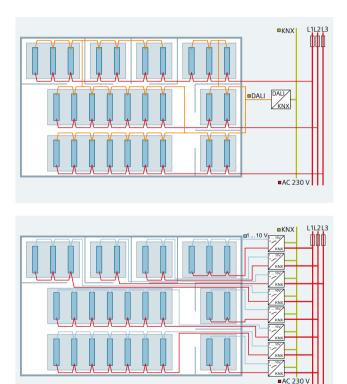
Modern lighting systems can be controlled efficiently and conveniently with DALI. Their efficiency can be increased even more when combined with the advantages of KNX. That's why KNX/DALI gateways from Siemens offer both standards directly: for DALI digital lighting (IEC 62386) and for KNX building control (ISO/ IEC 14543-3 or DIN EN 50090). It's possible to integrate DALI lighting into KNX installations quickly and easily.
