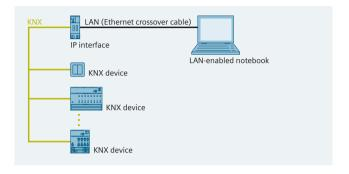
In every GAMMA instabus project, the devices are commissioned after their installation. Once the physical addresses have been assigned, application programs, parameters and addresses are loaded to the devices. This can take some time in large-scope projects with many devices.
