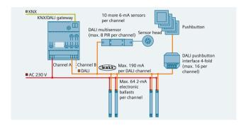
The KNX/DALI gateway can control up to 64 ballasts per channel. In addition, selected DALI sensors that meet specifications from Siemens can be commissioned together with the KNX/DALI gateway. The maximum number of DALI devices is limited to the guaranteed rated current of 190 mA per channel or to the maximum number of the DALI sensor type.
