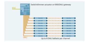
Ballasts with a DALI interface are used in lighting controls, e.g., to report lamp failure. The N 525E switch/dimmer actuator now makes it possible to completely replace DALI devices with GAMMA instabus without any knowledge of DALI or DALI commissioning procedures.
