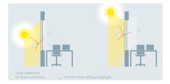
With sunlight tracking control, the position of the sun is tracked so that the blind slats are not completely closed, but rather automatically adjusted to prevent the sun from shining directly into the room. The spacing between the blind slats still allows diffuse daylight to enter the room and contribute to ensuring glare-free room lighting while lowering electricity costs.
