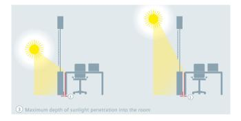
With shadow tracking control, sun protection is not lowered completely but only so far that the sun can still shine into the room for a certain distance (e.g. 50 cm), which can be set by adjustable parameters.
