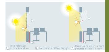
The functions of sunlight tracking control and shadow tracking control can be performed with the same devices individually or in combination.
